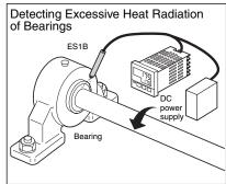
Do not use the Infrared Thermosensor in locations where the ambient temperature changes rapidly. To use the Infrared Thermosensor in locations subject to rapid changes in temperature due to radiant heat or movement of hot air, use a heat shield or other method to reduce rapid changes in temperature as much as possible.
